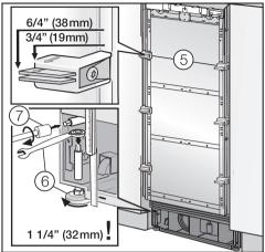
The installation aids (§) have been designed for the following total thicknesses of custom doors:
